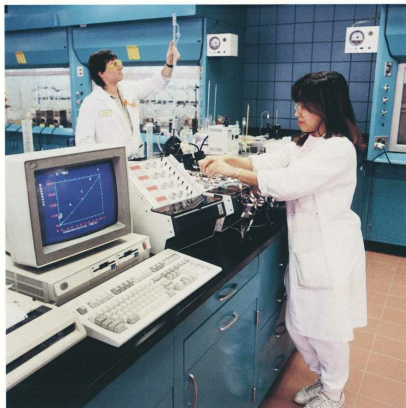
Laboratory analysis provides indicators on how well the District is treating wastewater and improving area water quality. Wastewater Analyst II Sandra Weeden and Wastewater Analyst I Mark Citriglia analyze wastewater for nitrogen ammonia, total Kjeldahl nitrogen, nitrate and nitrite.
