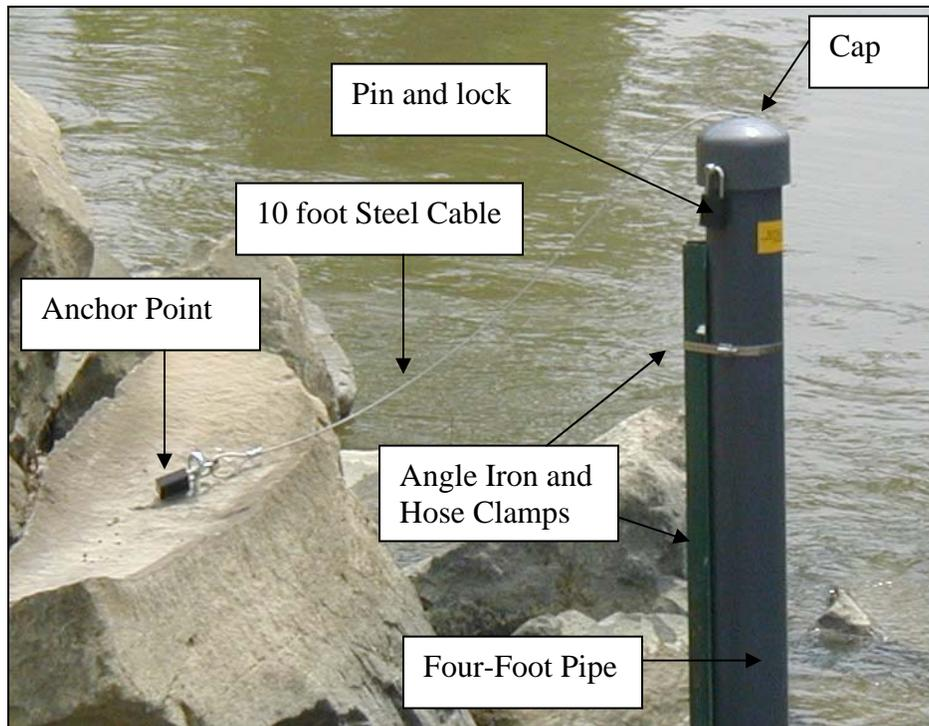
Figure 1. Data sonde installed in the Cuyahoga River
