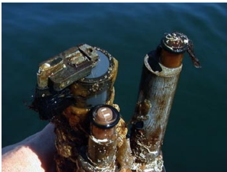
A prototype 6600EDS after continuous deployment for 80 days in Buzzards Bay, MA. The sensor in the foreground is the active DO sensor. The sensor at top-right was used as a non-wiped fouling reference. Note extensive fouling by plant and animal species on the non-wiped sensor.
