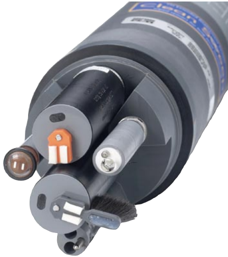
Profile of the 6600EDS depicting (clockwise from bottom) temperature/conductivity, turbidity, Rapid Pulse™ dissolved oxygen, chlorophyll and pH/ORP—all of which (except conductivity) are kept free of fouling by the patented Clean Sweep® universal wiper assembly, as well as individual optical wipers.
