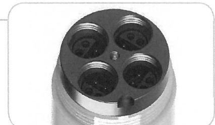
EXO1 sonde contains 4 universal sensor ports
