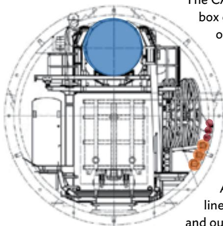
The CASSETTE (blue) is a box containing a flexible line of ventilation bag that reaches the length of the tunnel, up the shaft, and out to the surface. The cassette slowly feeds out the compressed bag as the TBM moves forward, providing air. Also pictured are water lines (orange) leading into and out of the tunnel alongside the A and B components of the grout mixture (red).
