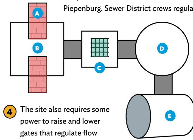
**2** The gate structure houses a set of angled screens that capture big debris, such as tires and tree trunks. “It’s easier to remove debris at a depth of 20 feet rather than hundreds of feet down,” says Mike Piepenburg. Sewer District crews regularly clean these screens.
