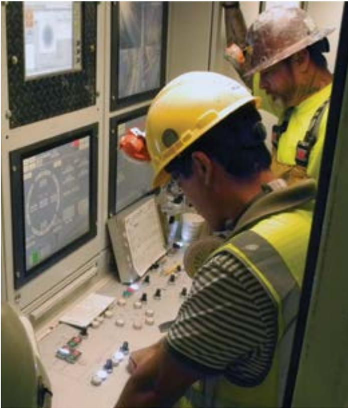
**Checking TBM progress from the Operators Cabin**
