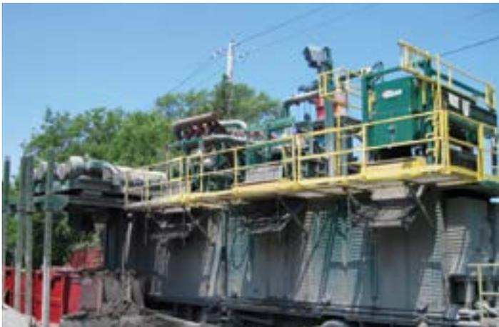
*The separation plant is where the excavated rock and soil is removed from the lubricant slurry.*
