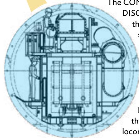
The CONVEYOR DISCHARGE is where the excavated shale from the cutter head empties from the overhead conveyor belt and into the muck cars to be carried out of the tunnel by the locomotive. □
