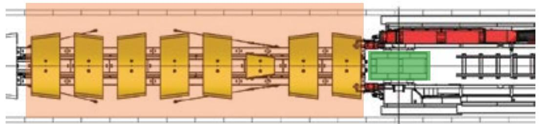
The ERECTOR can rotate a full 360 degrees to place the tunnel-lining segments, and it can also telescope towards and away from the cutter head.
