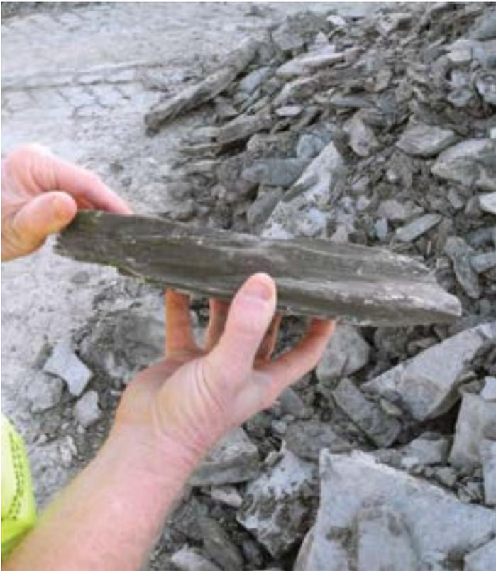
*Chagrin Shale is easy to mine and not very abrasive, which saves wear on the TBM.*
