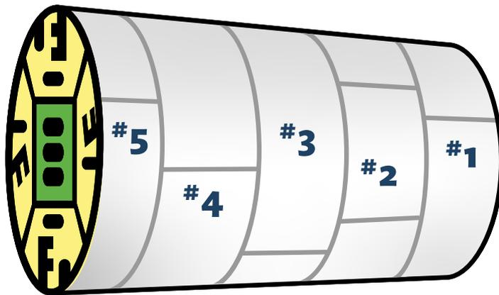
The TBM used on a project like the Doan Valley Tunnel places and grouts curved concrete segments to complete a ring (#1). Then the TBM pushes itself forward from that first ring and installs the next one, and so on.
