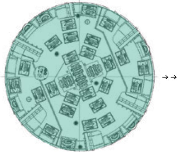
Mounted on the cutter head are discs of heavy-duty tungsten carbide steel that pulverize the shale. Each disc weighs over 250 pounds.
