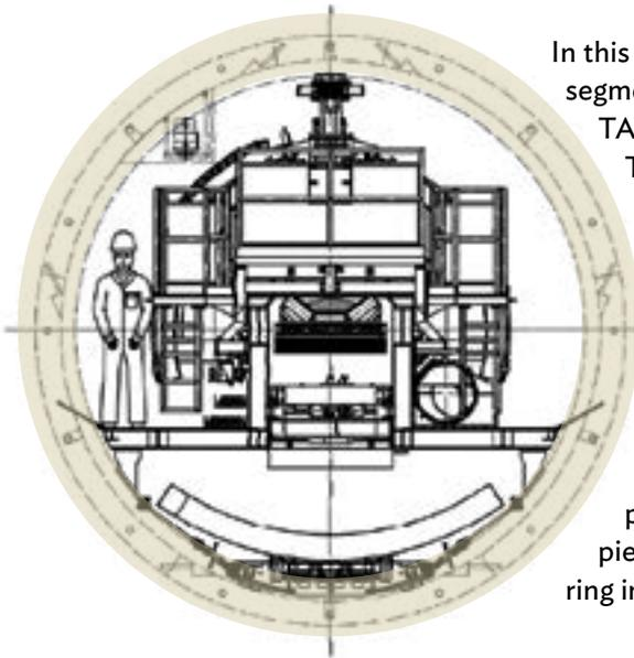
In this cross section, a tunnel segment sits on the SEGMENT TABLE awaiting placement. The segments are placed by the ERECTOR to make a complete ring (gray). Several of each segment can be stacked on tables. Working from the bottom, the erector builds up both sides and puts the small keystone piece on top, setting the ring in place.
