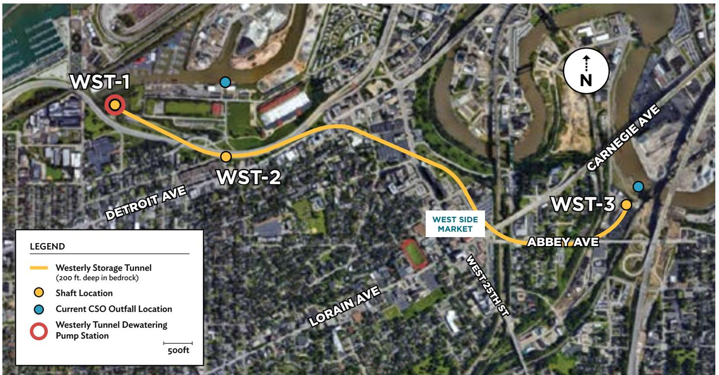
The tunnel boring machine began its journey at WST-3 and will exit the ground at WST-1 near the Westerly treatment plant.
