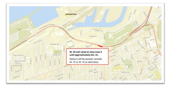
This ramp will temporarily close so the Northeast Ohio Regional Sewer District can continue construction of the <u>Westerly Storage Tunnel</u>. This project began in May 2018 and is the first tunnel on Cleveland's west side. This \$135 million project will capture 300 million gallons of combined sewage annually, preventing flows from entering the Cuyahoga River. The two-mile long tunnel runs beneath Tremont, Ohio City and Detroit-Shoreway neighborhoods.
