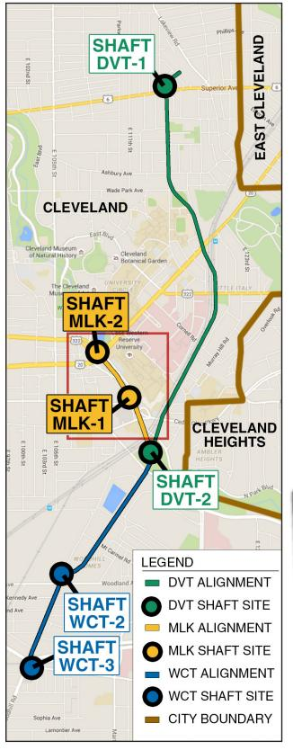
DVT project map, including all three tunnel segments (DVT, MLK, and WCT) and six tunnel shafts. The area in the red box is shown in more detail on the next page.
