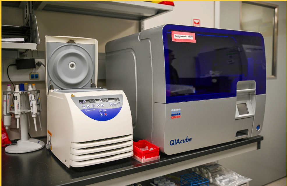
The lab's DNA-extraction workstation. The Qiacube (right) can automate DNA extraction, and its centrifuge feature makes the manual extraction process easier. A refrigerated centrifuge (left) keeps samples cool during the initial steps of extraction.
