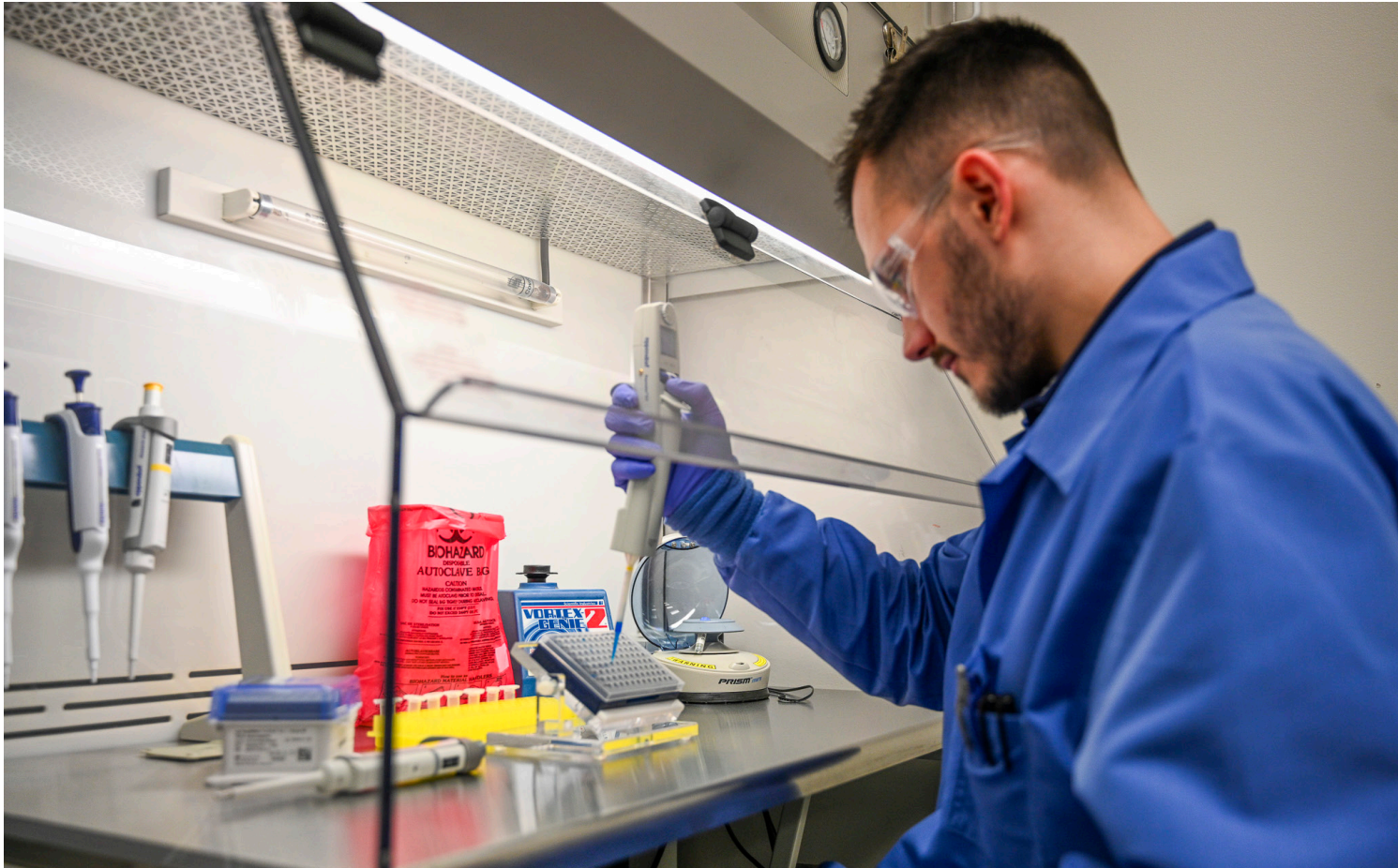
Lab Analyst Matt Lauren prepares a water sample using an auto pipettor. Auto pipettors are designed to deliver very small volumes of liquid and are checked for proper operation daily.
