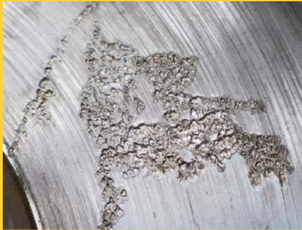
Cavitation damage on a pump casing (Photo courtesy of Central States Industrial)
