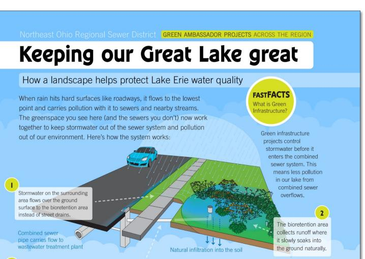
When the storm exceeds the bioretention area's capacity, excess runoff is conveyed to the street sewer system, which drains to the combined sewer system.
