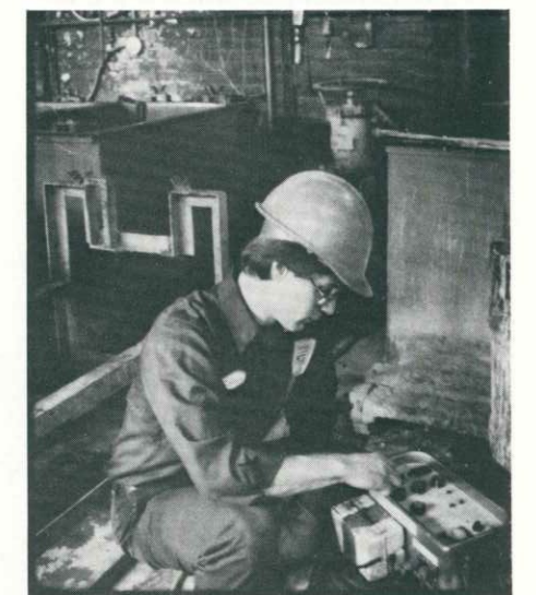
As part of the District's industrial pretreatment program, Frank Schuschu, investigator for the Industrial Waste section, adjusts a device placed at an electroplating company to sample the discharges from that facility.
