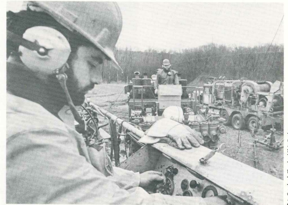
At the natural gas well site, located on the grounds of the Southerly Wastewater Treatment Plant, a technician monitors the fracturing process which cracks the sandstone into which the well is sunk.
