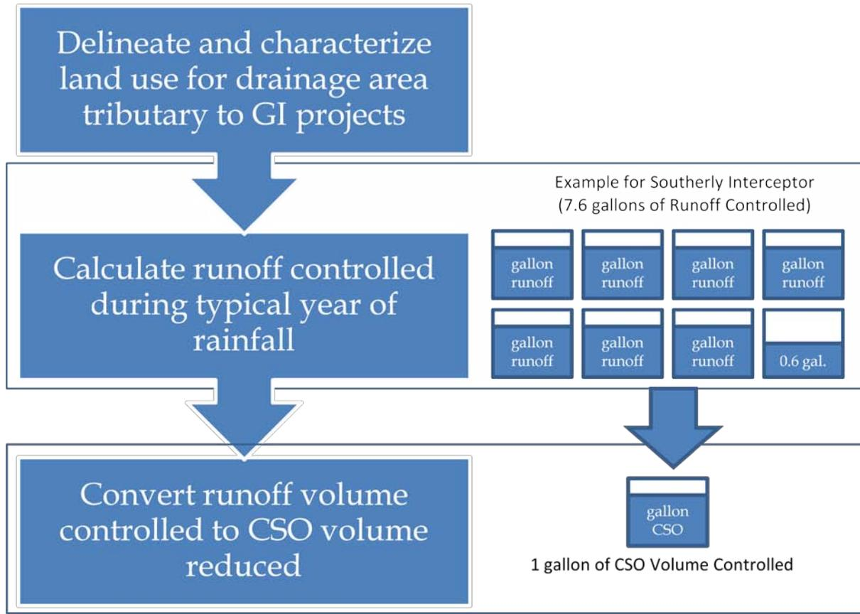
Figure 13. Process to Calculate CSO Volume Reduction Potential for Each GI Project
