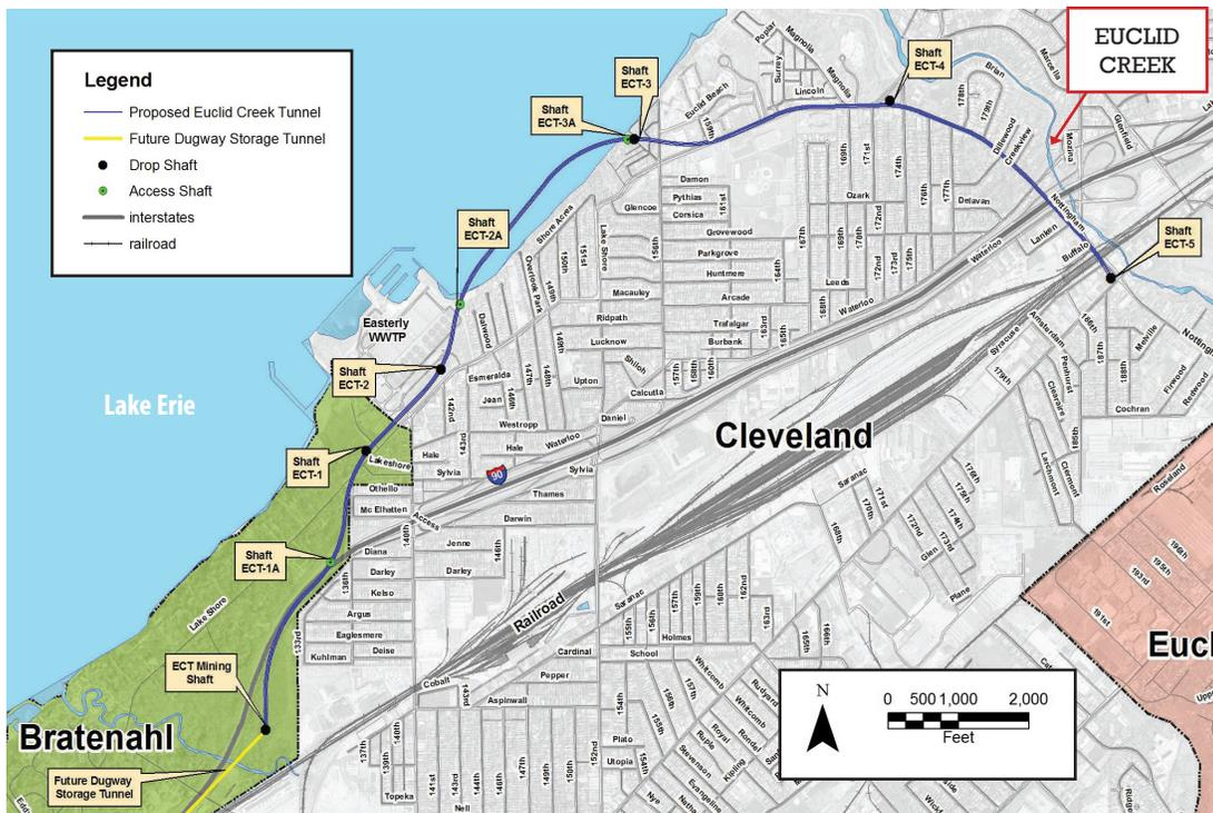
Tunneling for this project will occur 190-220 feet below ground and residents will only see construction equipment at six street-level shafts.
